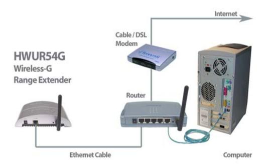
You may also connect the HWUR54G to an open LAN port on your network. After you have finished configuring your Range Extender (the following steps will help you configure your Range Extender) you must disconnect it from your network or PC and place it in any location that requires extended wireless coverage (must still be in wireless proximity of your original wireless network):
